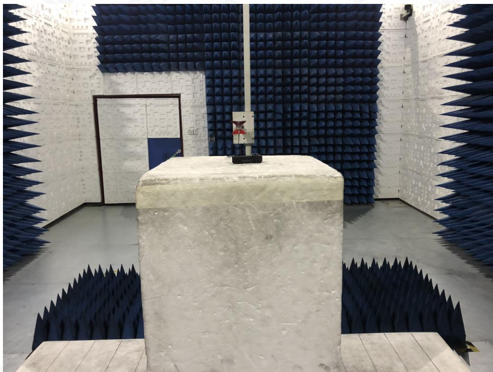
FCC RADIATED EMISSION TEST SETUP ABOVE 1GHZ
