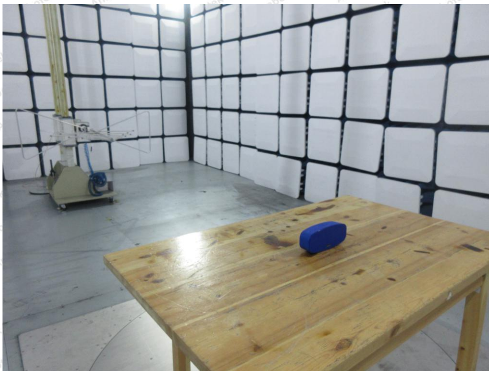
Photo of Radiation Emission Test
