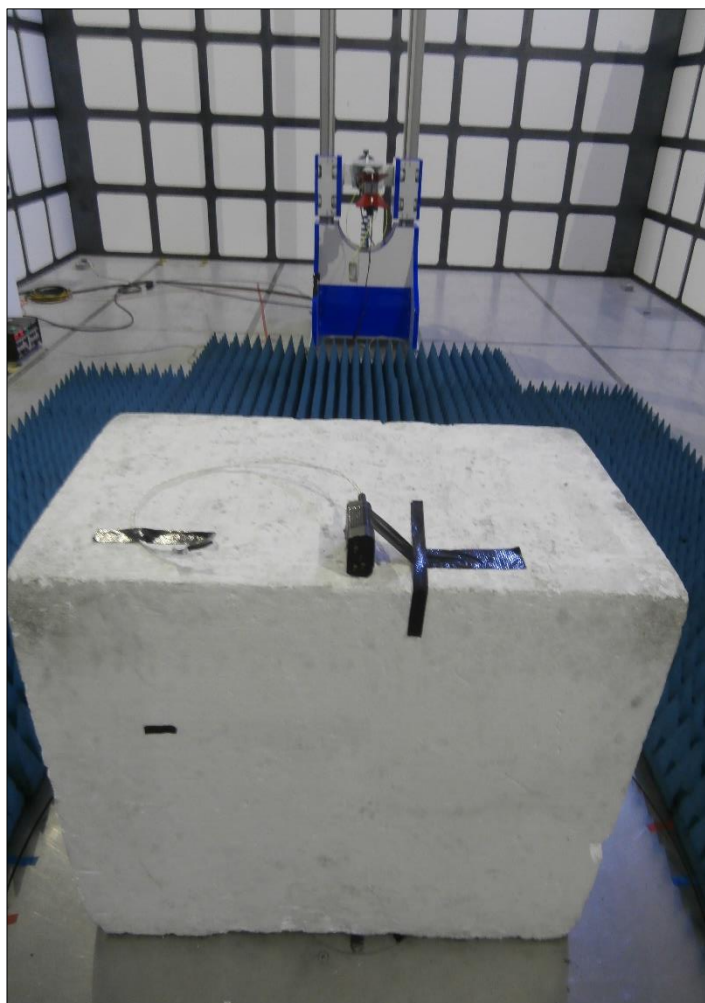
Figure 25 – Test Setup 1 GHz to 13 GHz - Z Orientation
