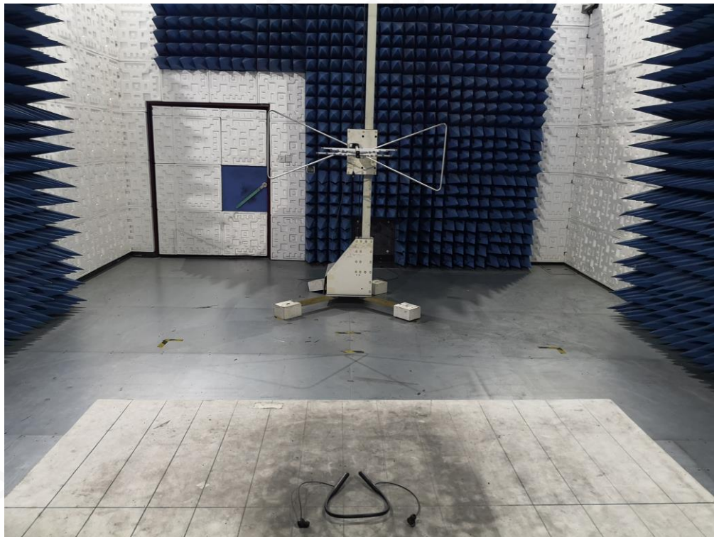
RADIATED EMISSION TEST SETUP ABOVE 1GHZ
