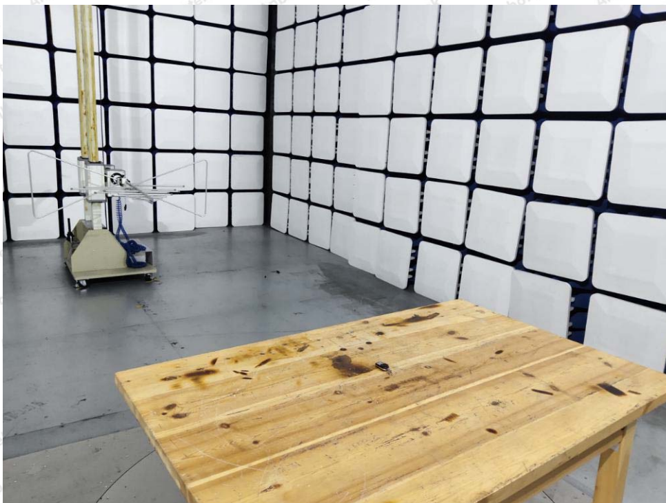
Photo of Radiated Emission Measurement
