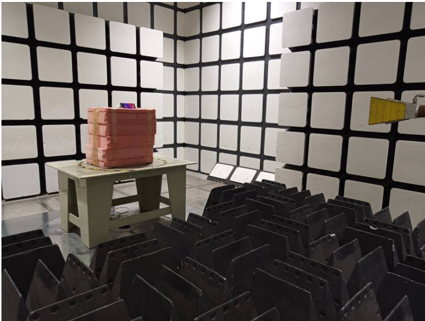
Radiated Emissions View (Above 1 GHz)
