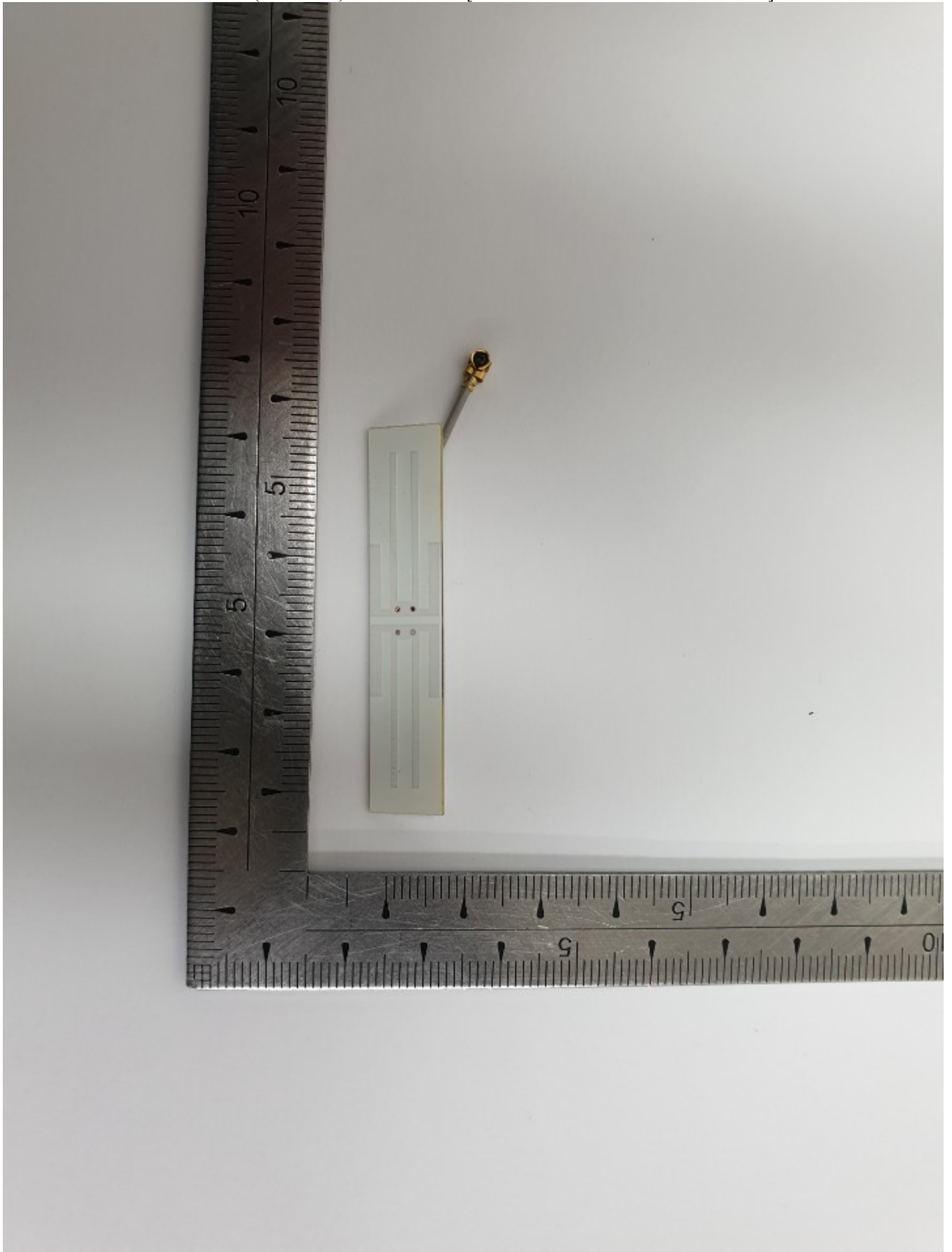
Antenna 2 (Additional) / PCB Antenna [Model name: AEi-2450/5500P-IPEX35]
