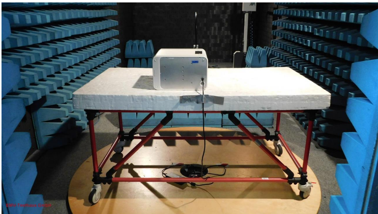
Picture 1: EUT test setup radiated emission test 9 kHz – 30 MHz (front view)
