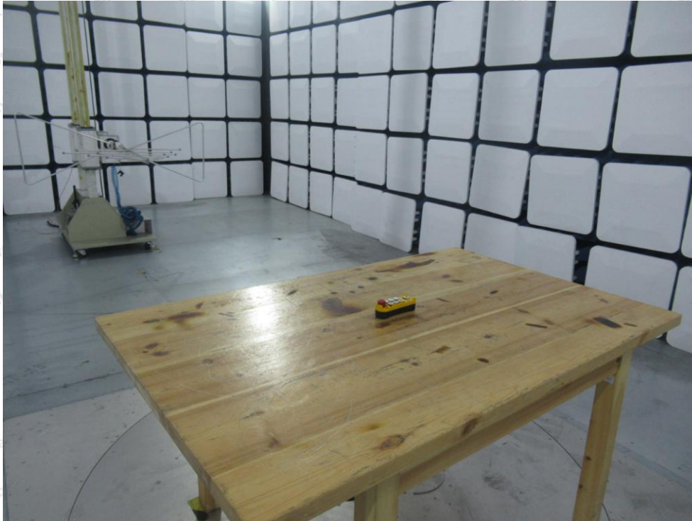
Photo of Radiated Emission Measurement
