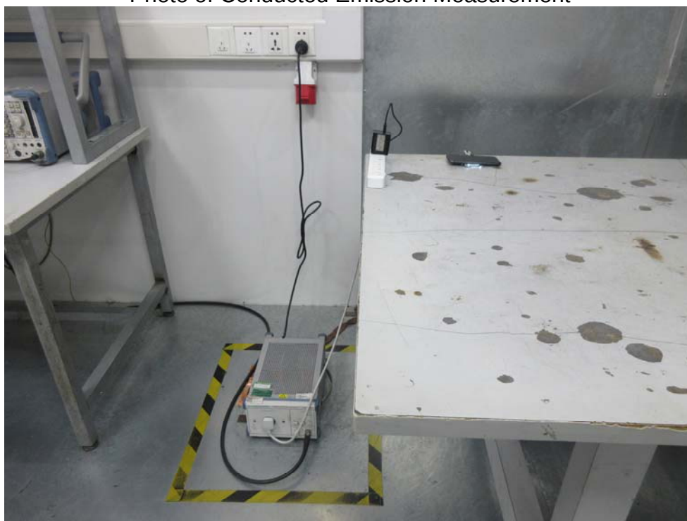
FCC ID: 2AVG8-LAMXON15 Photo of Conducted Emission Measurement
