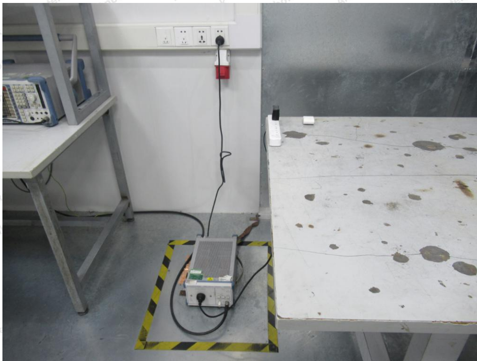
Photo of Conducted Emission Measurement
