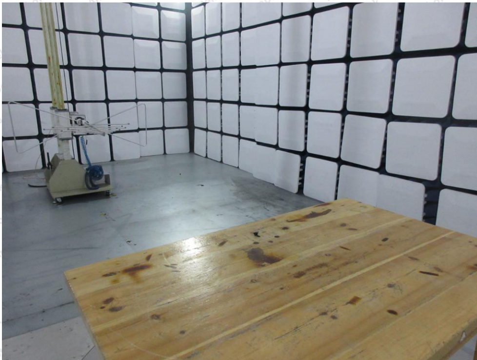
Photo of Radiation Emission Test
