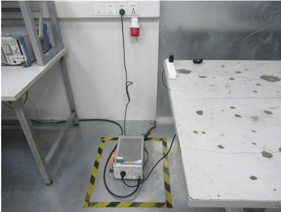
Photo of Conducted Emission Measurement
