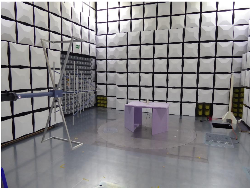
191836_02.JPG: Setup SAC E-field
