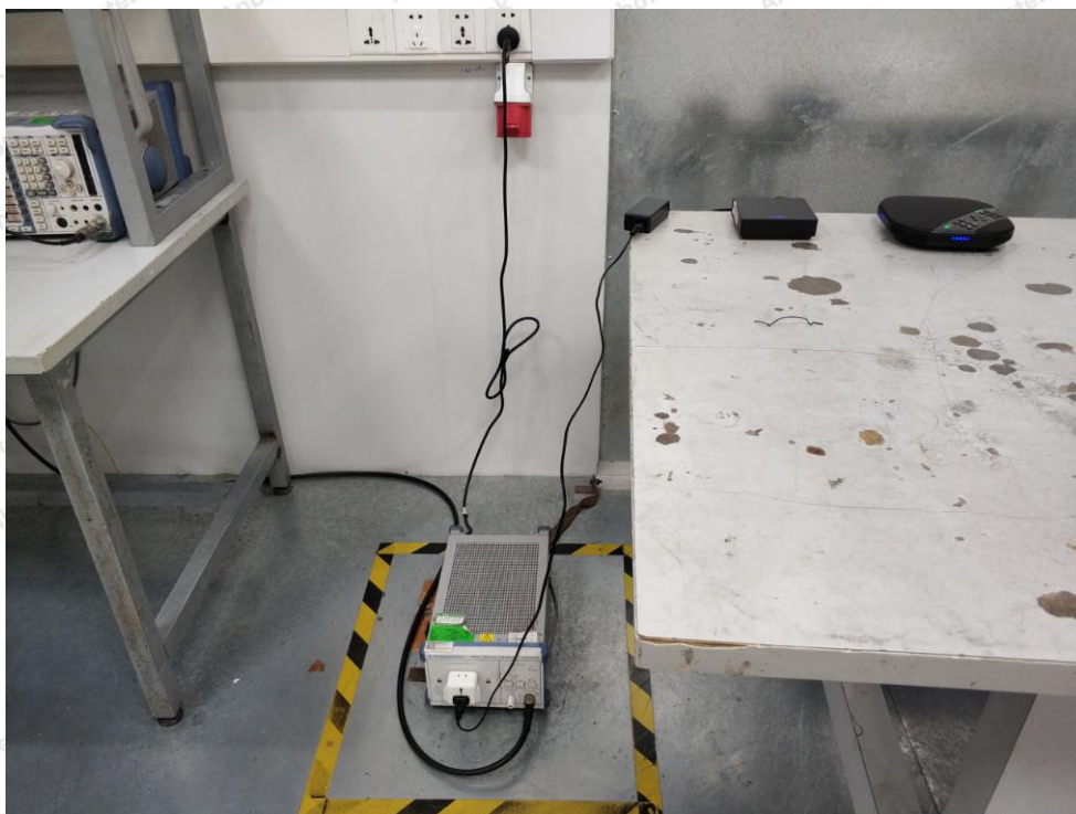
Photo of Conducted Emission Measurement
