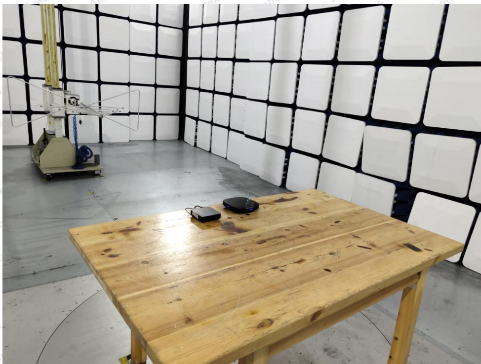
Photo of Radiation Emission Test
