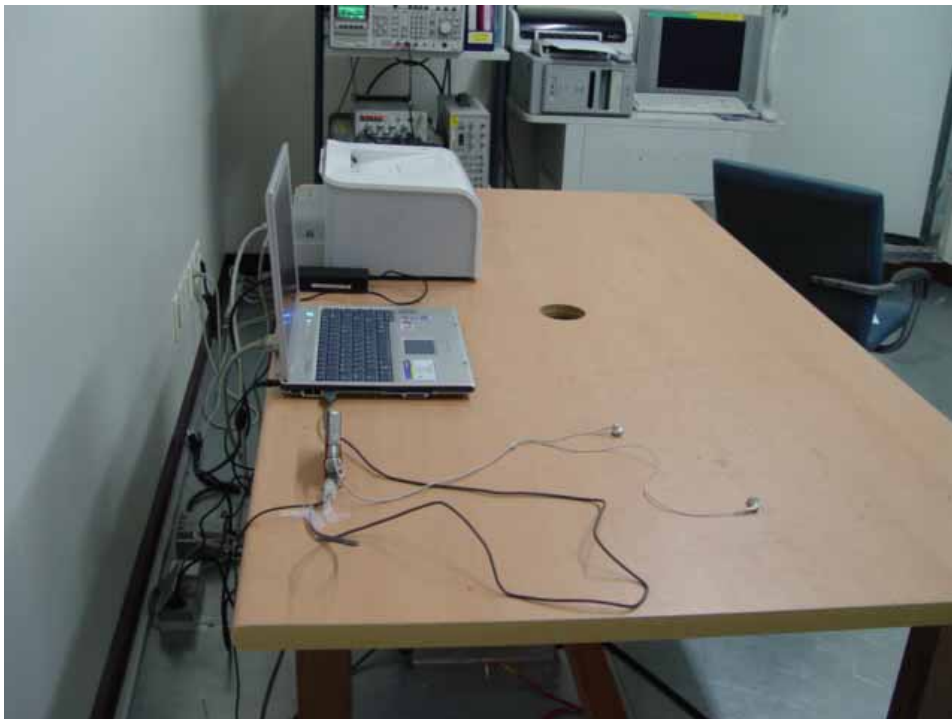
Picture 2. Conducted Emission (Side)
