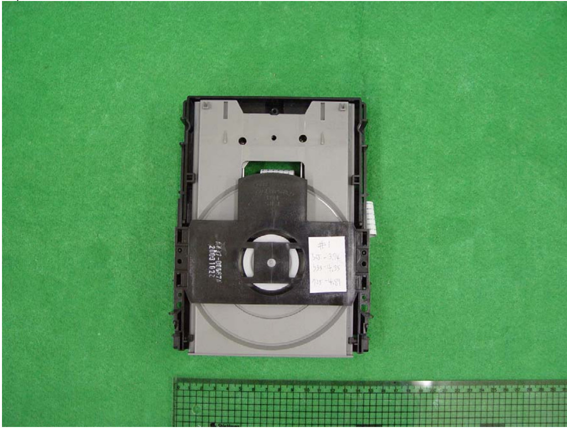
Bottom of DVD Deck Mechanism View
