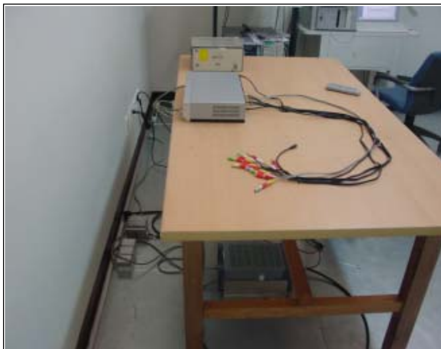
Pic. 2 AC Powerline Conducted Emission [Rear]
