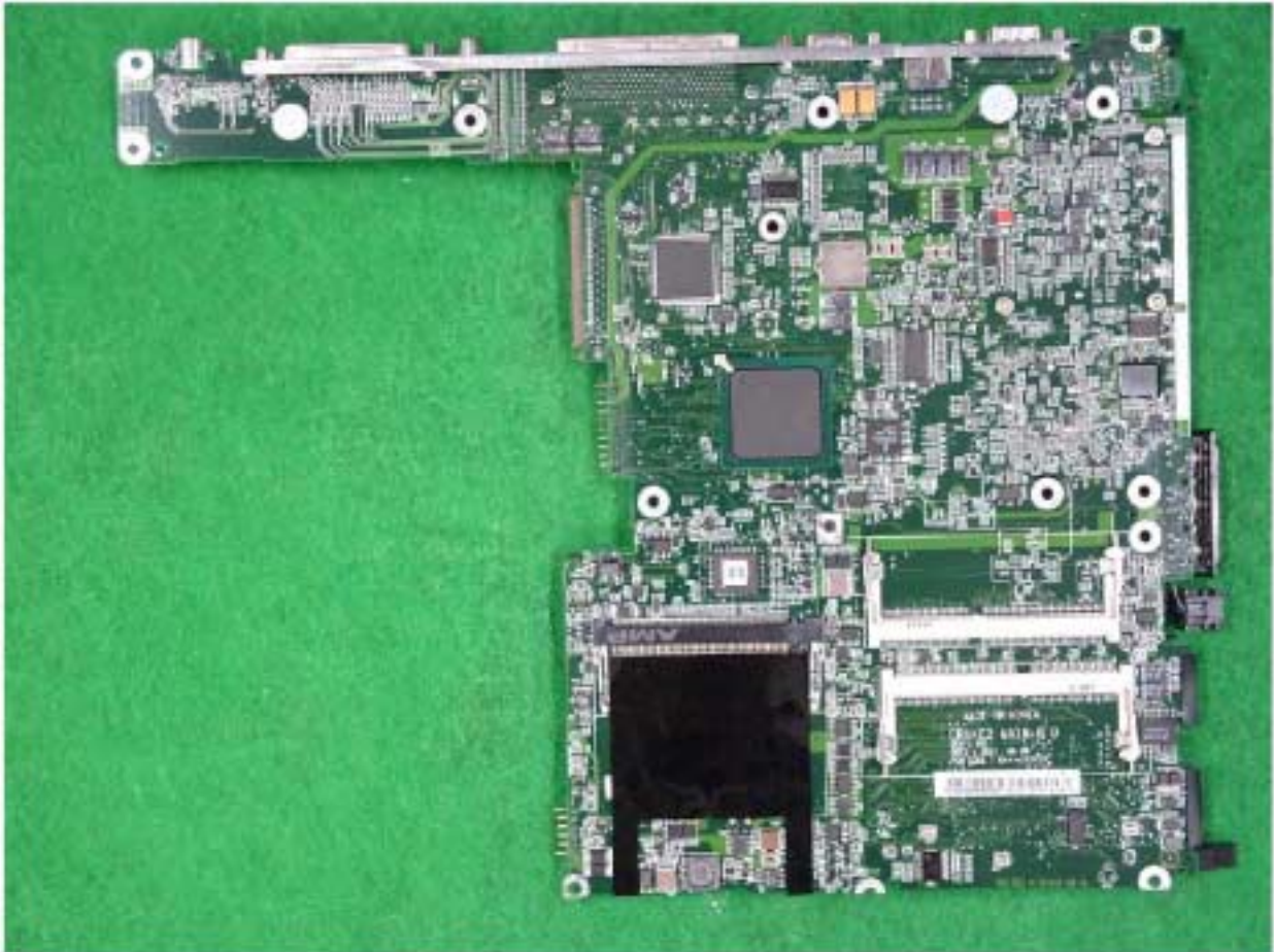
PHOTOGRAPH 6-7: TOP VIEW OF THE BOARD WITHOUT CAN
