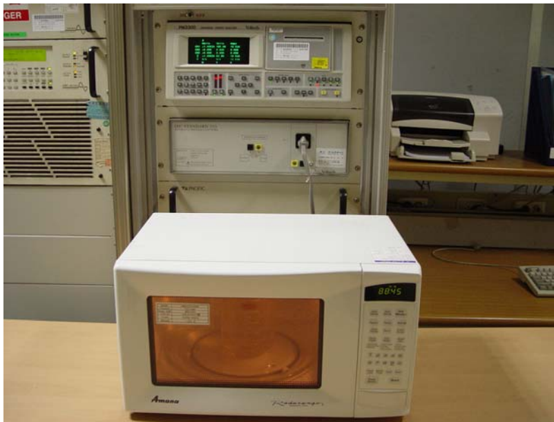
Fig.3 Test Setup for RF output power
