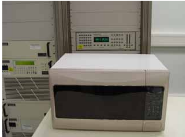
Fig.3 Test Setup for RF output power
