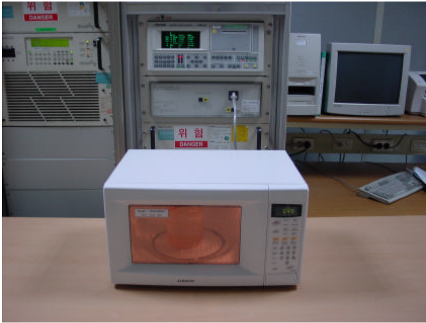
Fig.3 Test Setup for RF output power
