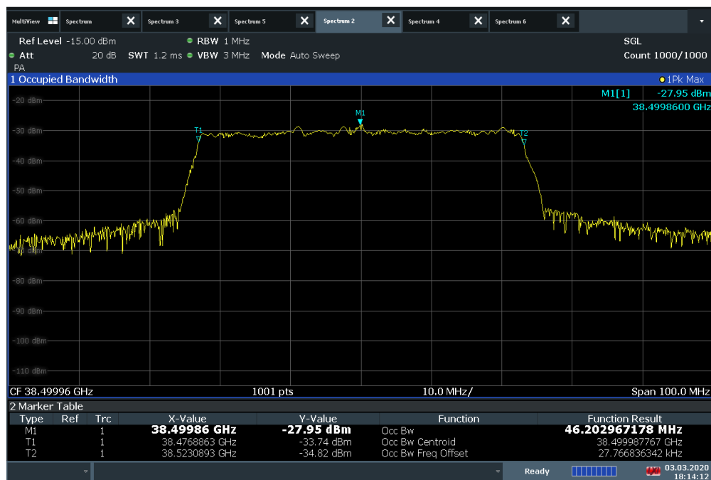
Plot 7-38. Occupied Bandwidth Plot (50MHz BW 1CC 16QAM Mid Channel)
