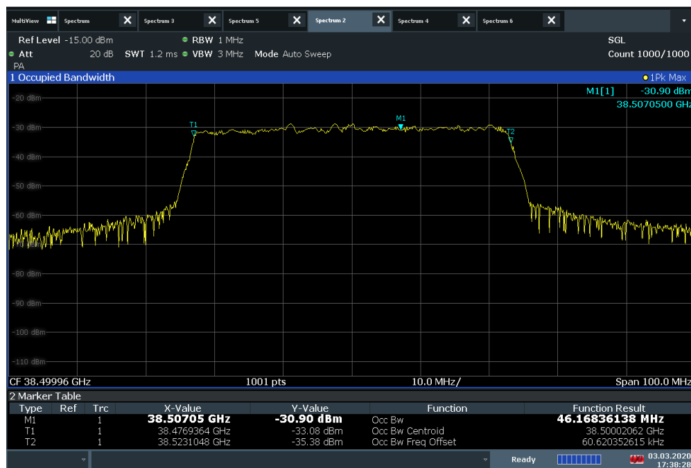
Plot 7-26. Occupied Bandwidth Plot (50MHz BW 1CC 16QAM Mid Channel)
