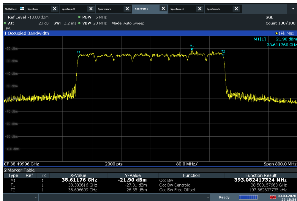
Plot 7-44. Occupied Bandwidth Plot (50MHz BW 8CC 16QAM Mid Channel)
