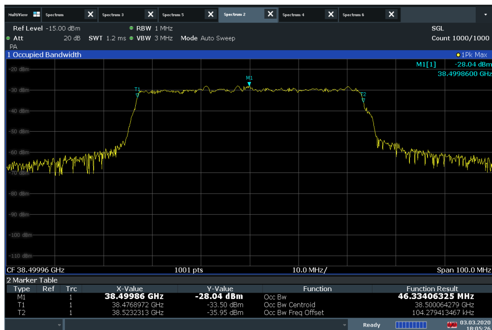
Plot 7-15. Occupied Bandwidth Plot (50MHz BW 1CC 64QAM Mid Channel)
