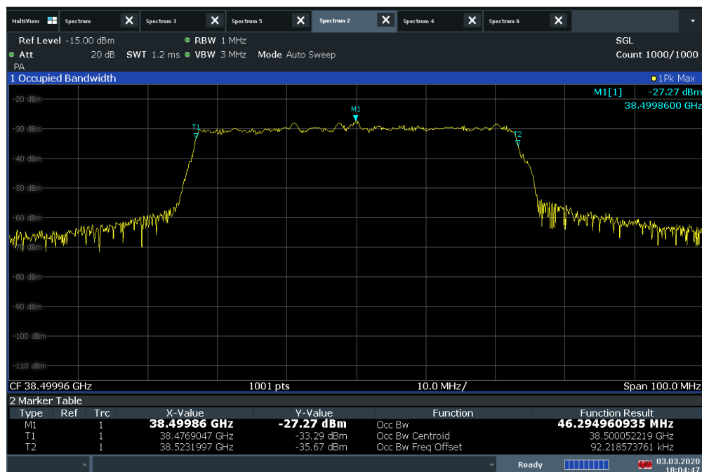
Plot 7-14. Occupied Bandwidth Plot (50MHz BW 1CC 16QAM Mid Channel)
