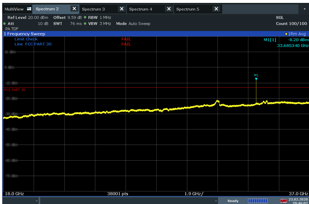
Plot 7-356. Radiated Spurious Plot 18-37 GHz (8CC NC QPSK High Ch. Ant. Angle 45, Final)
