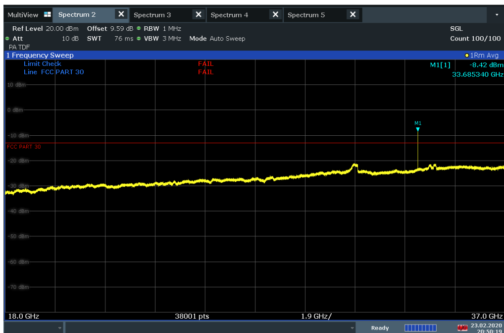
Plot 7-354. Radiated Spurious Plot 18-37 GHz (8CC NC QPSK High Ch. Ant. Angle 135, Final)
