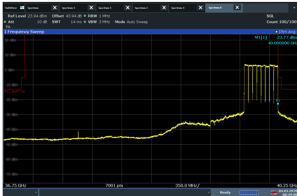
Plot 7-509. Band Edge Plot (50MHz BW 8CC QPSK High Channel)
