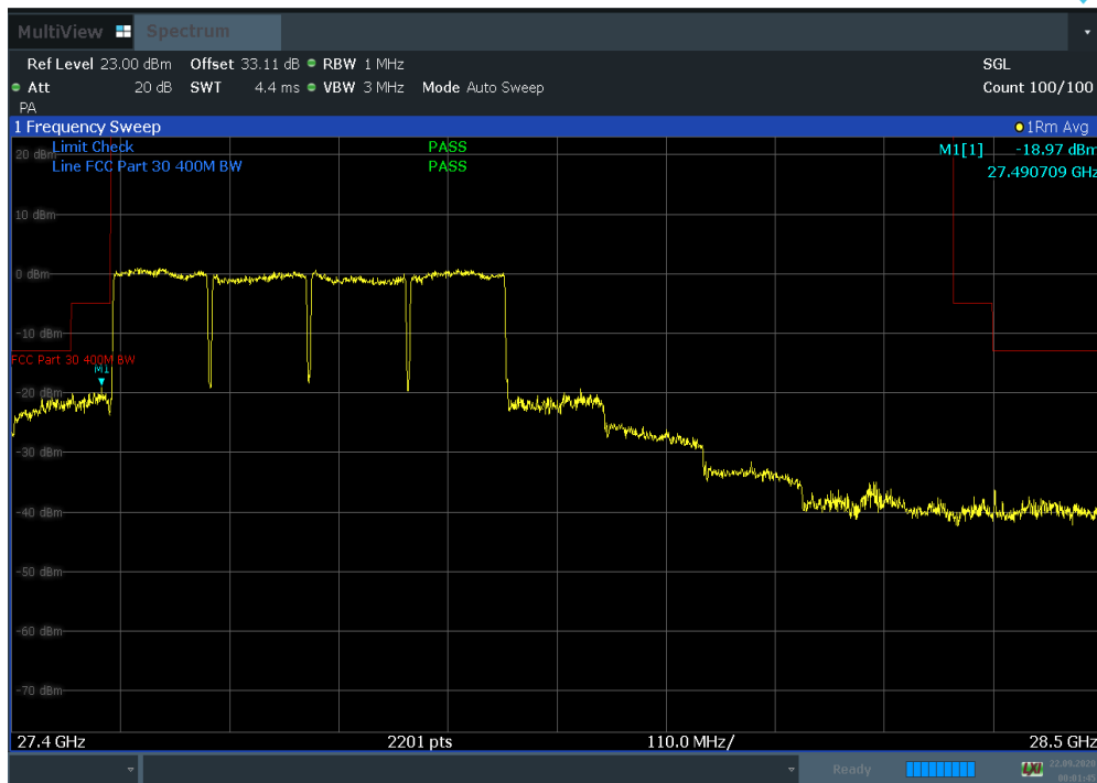
Plot 7-745 Band Edge (Ant C 100 MHz BW 4CC CC QPSK Low)
