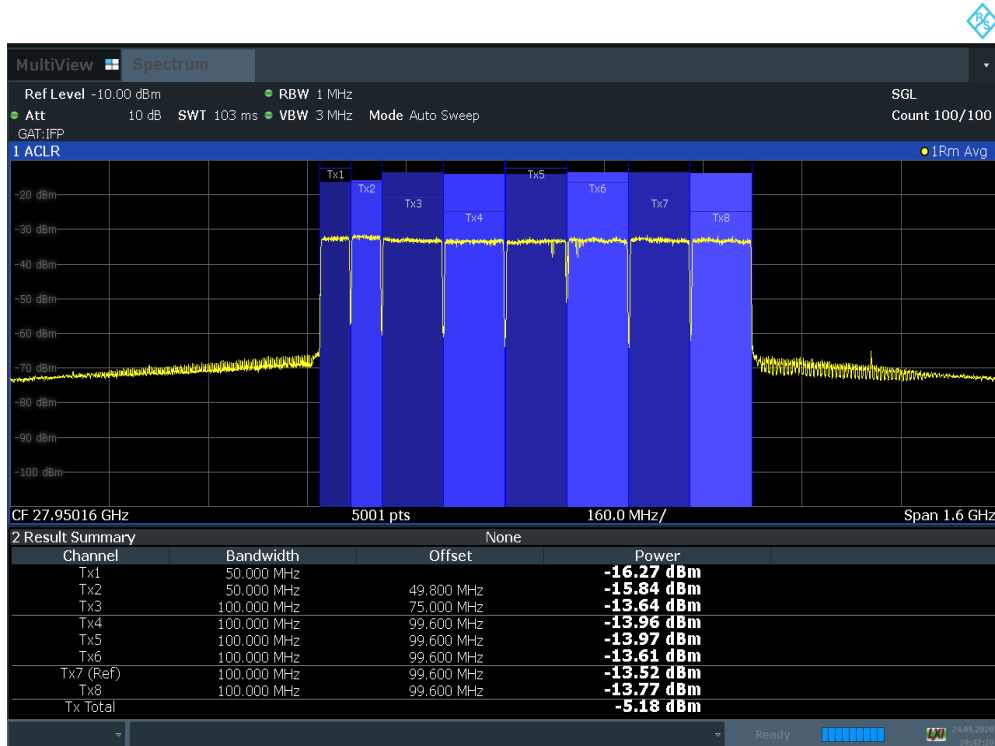
Plot 7-264. EIRP Density (Ant D 50 MHz 2CC + 100 MHz BW 6CC QPSK High)
