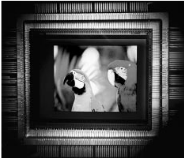
Figure 46. DMD front projection display showing entire chip area (768 x 576 array, 640 x 480 image).
