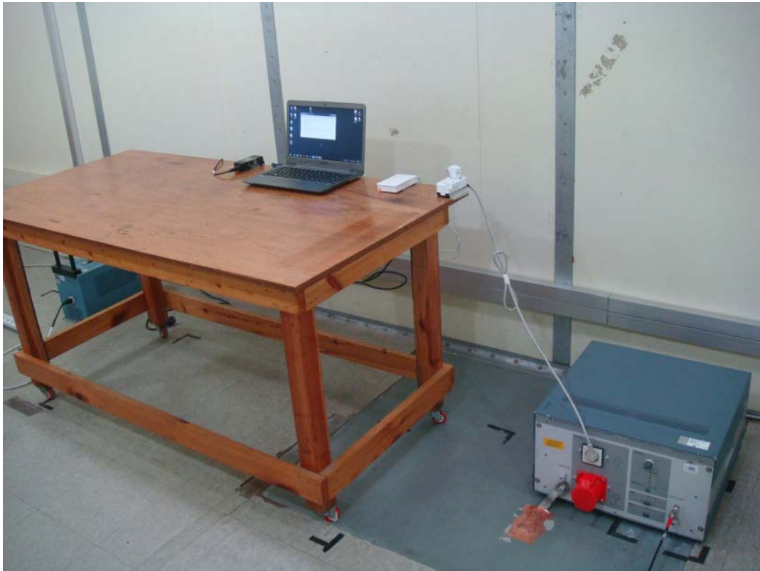
AC Power line conducted emissions - rear view
