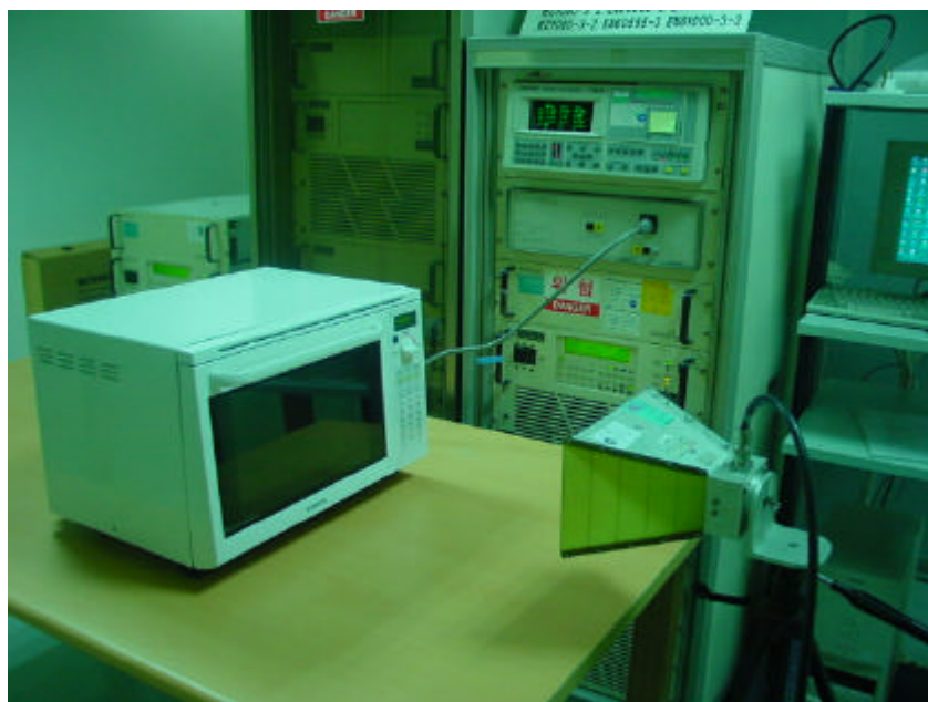
Fig. 2 Test Setup for Input power
