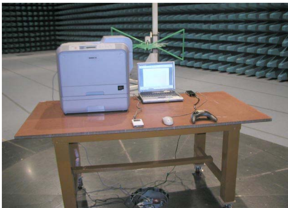
Pic. 3 Radiated Emission (Front)
