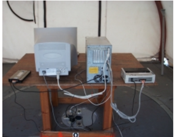
Radiated Emission Setup Photos (Worst Emission Position)
