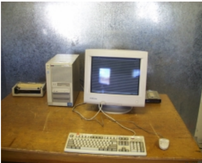
Conducted Emission Setup Photos (Worst Emission Position)
