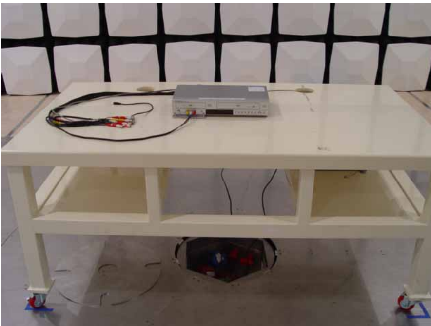
Picture 2. Radiated emission (Front)
