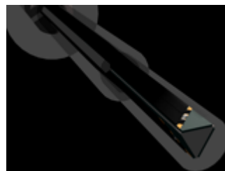
Figure 4-3 Triangular Probe Configuration
