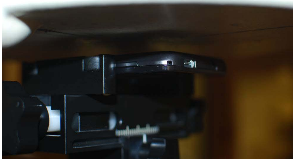
Figure 21-5 SAR Test Setup Photo 5 – Back at 1.0 cm
