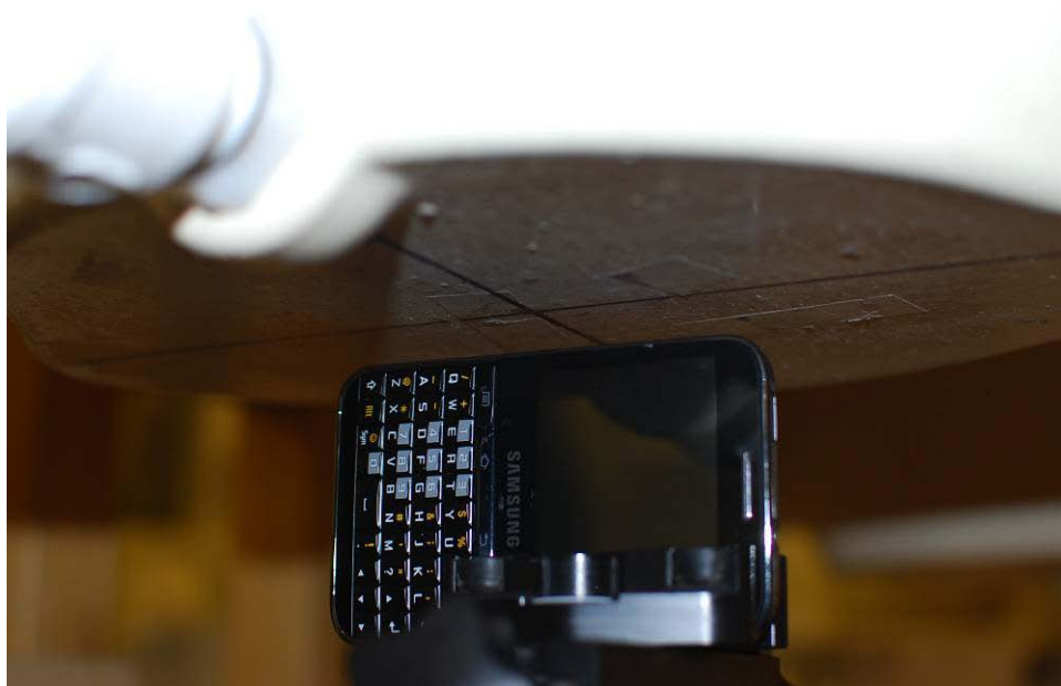
Figure 21-10 SAR Test Setup Photo 10 – Left at 1.0 cm
