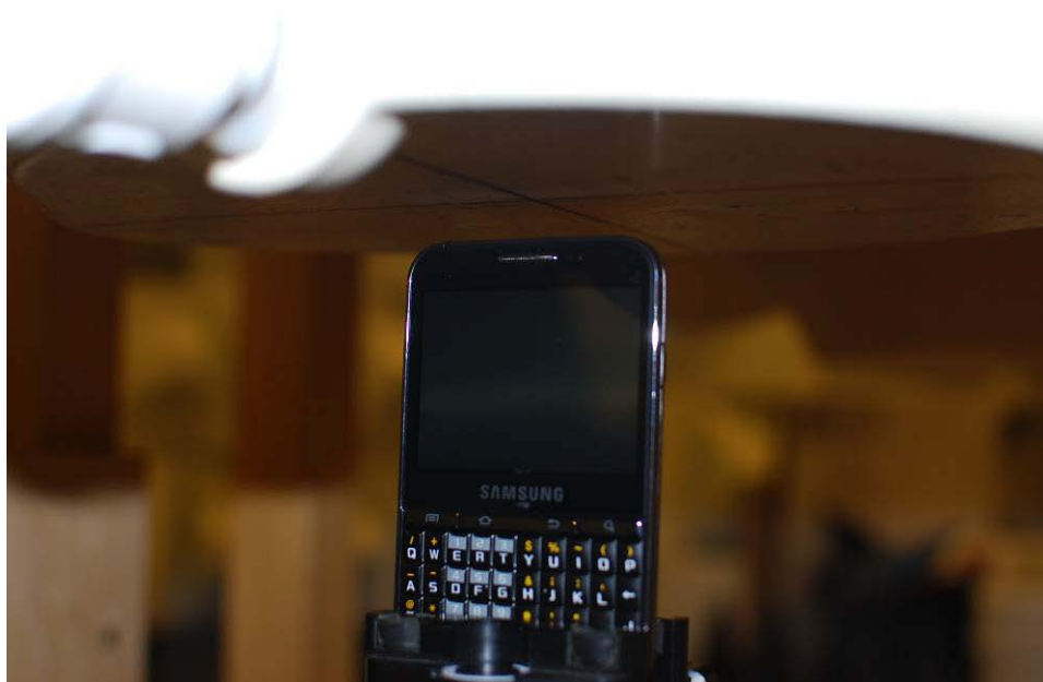
Figure 21-7 SAR Test Setup Photo 7 – Top at 1.0 cm
