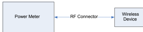
Figure 14-1 Power Measurement Setup
