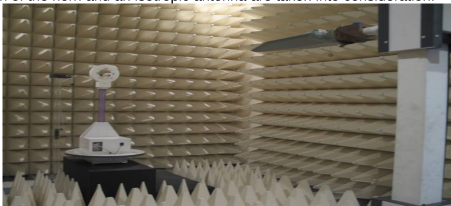
Figure2. Photograph of 3m Fully-Anechoic Chamber
