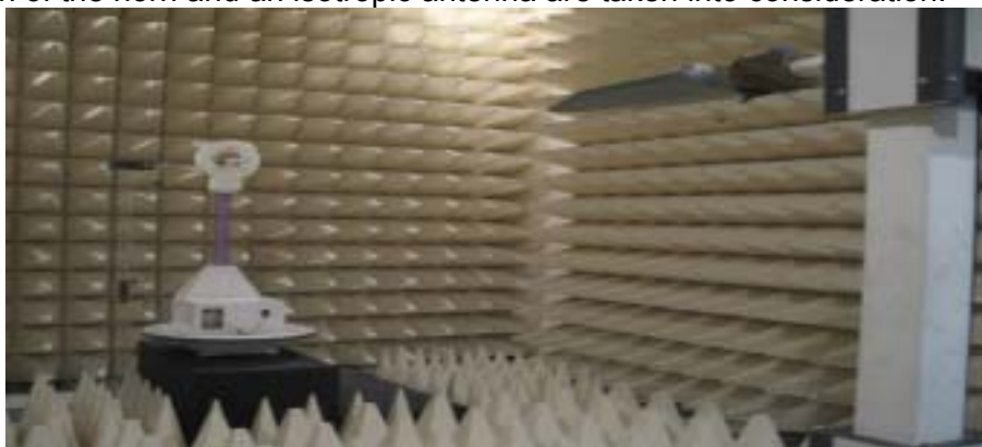
Figure2. Photograph of 3m Fully-Anechoic Chamber
