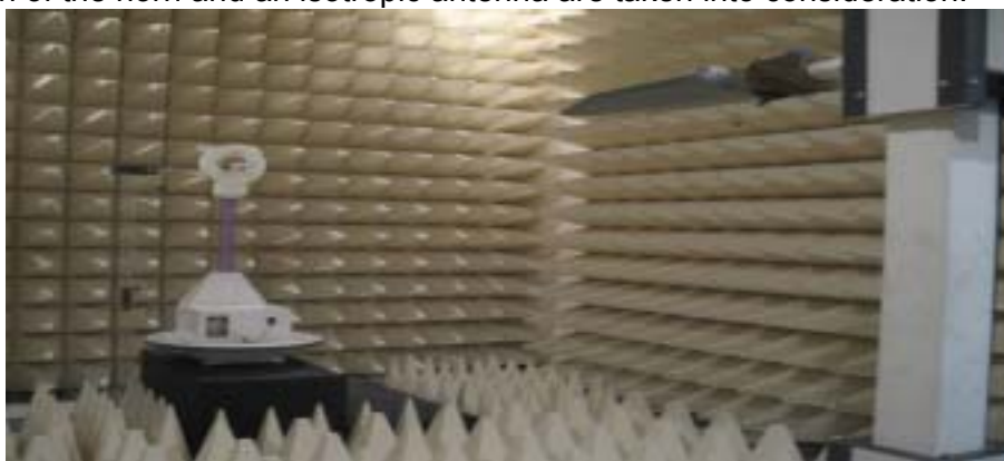
Figure2. Photograph of 3m Fully-Anechoic Chamber
