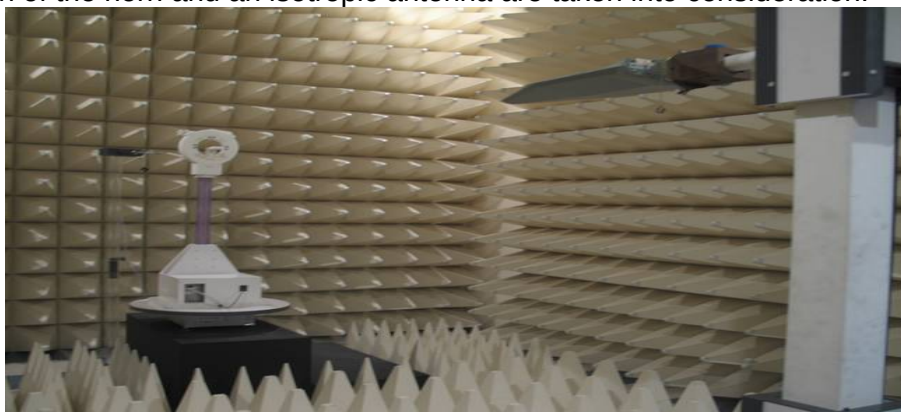
Figure2. Photograph of 3m Fully-Anechoic Chamber
