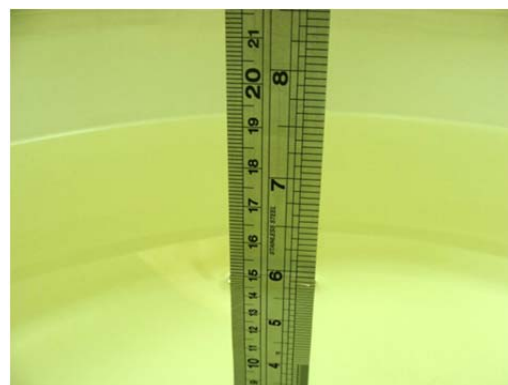
Fig 6.2 Photo of Liquid Height for Body SAR
