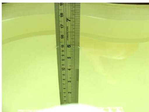
Fig 6.1 Photo of Liquid Height for Head SAR
