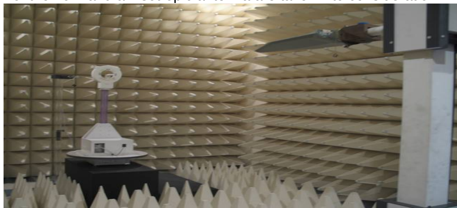
Figure2. Photograph of 3m Fully-Anechoic Chamber
