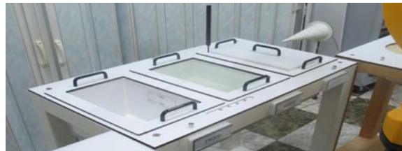
Figure 3.6 Modular Flat Phantom
