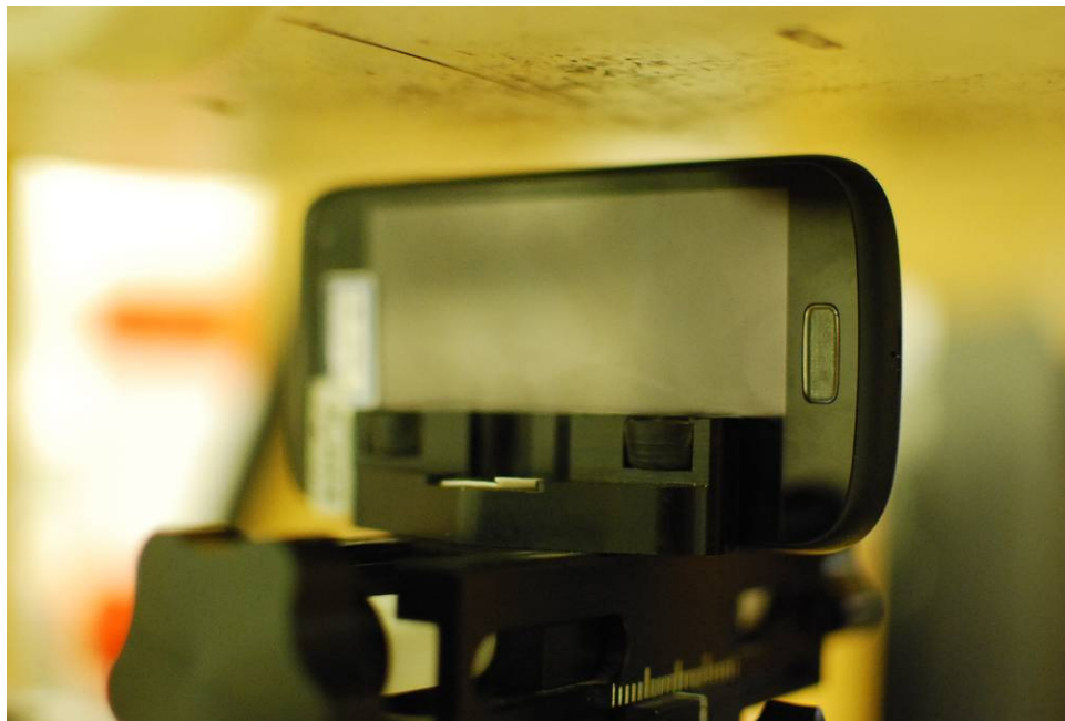
SAR Test Setup Photo 8 – Right at 1.0 cm
