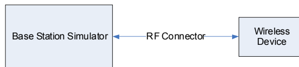
Figure 9-1 Power Measurement Setup
