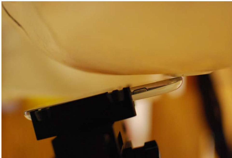
SAR Test Setup Photo 4 – Left Tilt
