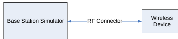
Figure 8-2 Power Measurement Setup
