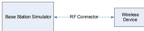
Figure 8-1 Power Measurement Setup
