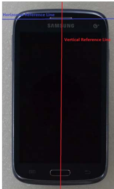
SAR Test Setup Photo 11 - DUT Horizontal and Vertical Reference Lines
