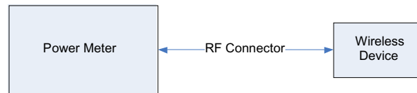
Figure 14-2 Power Measurement Setup
