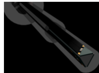
Figure 4-3 Triangular Probe Configuration
