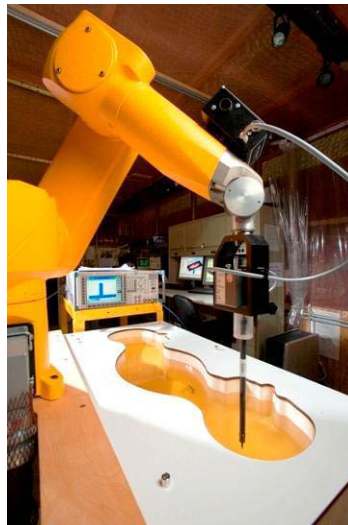
Figure 3-2 DASY4 SAR Measurement System
