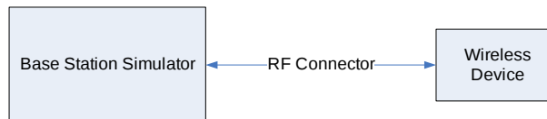
Figure 11-1 Power Measurement Setup
